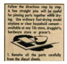
This plan package is not die-cut like the original kit. It is highly recommended that a sharp Xacto® blade be used at all times. Don't skimp on this or you will tear the wood when cutting it out. Off-brand blades are not as good as the Xacto® brand. When the blade starts to drag, change it out for a new one. It is also best to **NOT** cut on the lines. Cut the pieces out oversized and sand down to the line. This is especially important when cutting out notches.
