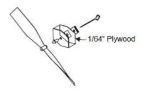
For the removable nose piece assembly, use the printed piece as a pattern to make up a backing piece from 1/64" plywood. A Peck thrust bearing for a 1/32" prop shaft is recommended. Use a prop in the  $5\frac{1}{2}$ " range. Installation of the rubber motor is made possible by an access hole in the fuselage bottom just below the motor peg.
