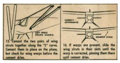
The struts in this plan package are assembled the same but attach to the wing differently. Instead of fitting into slots in the wing, attach the struts to the inboard side of the rib that was attached near the aileron in the previous step. Before gluing into place, the struts can be trimmed to correct any wing warping.
