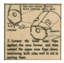
As mentioned in the previous step, this plan package has a one-piece top and bottom cowl. Since they are made of 1/32" balsa they should bend to shape the nose without moistening.
