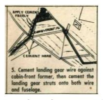
A two-part epoxy cement works best here. Super Glue will work if desired and will keep the plane light. Another option is to cover the gear where it attaches to the cabin former with scrap balsa.
