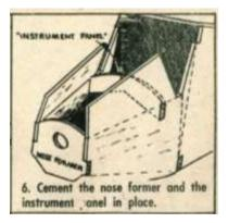
The original kit had each half of the nose cowl included as part of each fuselage side. This has been replaced with a one-piece top and bottom cowl that are oversized so they can be trimmed to fit. The nose former provided in this plan package is intended for a removable nose piece.
