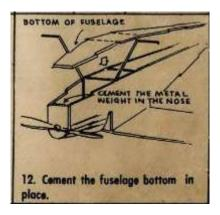
It shouldn't be necessary to moisten the nose bottom. If it is, moisten the bare side, not the printed side.
