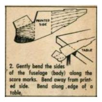
This step was necessary because the original kit used 1/16" balsa. Since this plan package uses 1/32" balsa, **DON'T** try to bend the sides prior to assembly. The 1/32" balsa will form to the contour just fine.
