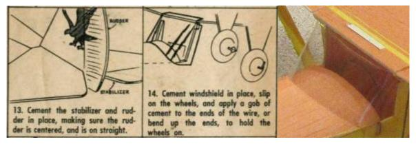
Step 14 shows the windshield glued on top of the wing. Since this plan package has a different wing arrangement, attach the window to the underside of the wing center section. The sides attach as shown. The original kit came with 3/4" wheels.
