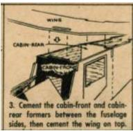
When gluing the front and rear cabin formers in place, lay one side of the fuselage on a flat surface. Brace the formers with something that will hold them at 90 degrees (straight up) and then add cement. When dry, attach the other half of the fuselage as shown.
