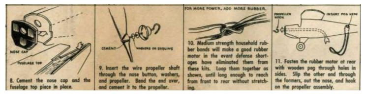
The fuselage top can be attached but only do the other steps if you will NOT be using a removable nose piece. When dry the edges of the fuselage top can be sanded flush to the sides.
