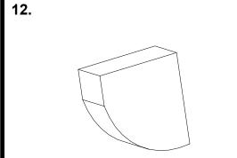
Cut out the launch hook from a piece of 1/8 inch thick aircraft plywood.
