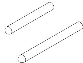
Cut a 1 1/2" and 2" length of dowel. Round off one end of each dowel as shown.
