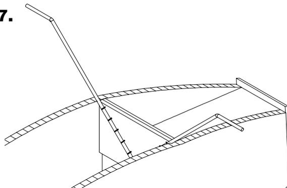
Glue F2A with the attached landing gear legs to the back side of F2. Line up the bottom with the bottom of F2.
