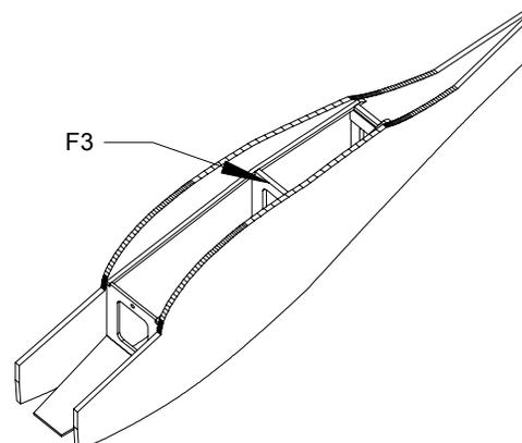
Glue fuselage former F3 in place. Again, use the drawn reference lines as a location guide.
