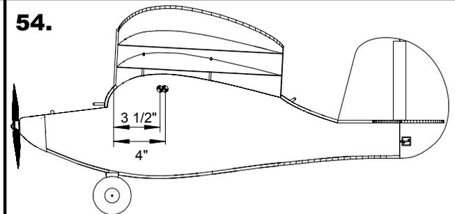
With your flight battery pack in place, check the Center of Gravity (CG) location. It should be in the range of 3 1/2 to 4 inches back from the wing leading edge. Your Lo 'N Slo is now ready for flight. Control throws are not critical.
