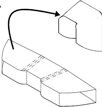
Cut the cowl from aluminum drink can stock using the supplied template. A good way to do this is to rubber cement the template to the aluminum sheet stock. Use the bend lines on the template to bend the cowl to the shape of F1.
