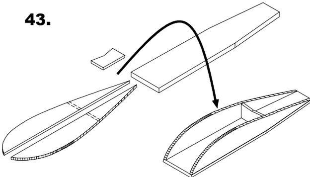
Mark each rib W1 with the location of CS1 using the printed template as a guide. Assemble the center section base structure as shown. Glue the ribs W1 to the top side of the base piece. Sand the leading edge of the base piece to match the rib profile.
