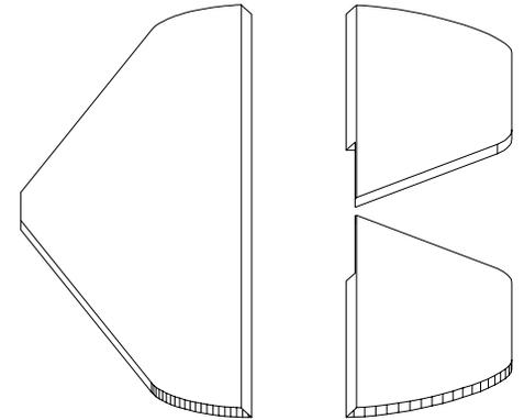
Sand the trailing edge of the stab so it is beveled as shown on the plan. Also sand the elevator leading edges to a bevel as shown on the plan.
