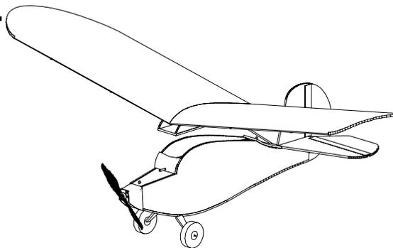
The wing assembly fits inside the fuselage sides behind fuselage part F5. Use several rubber bands to retain the wing assembly. The rubber bands are looped around the two dowels.
