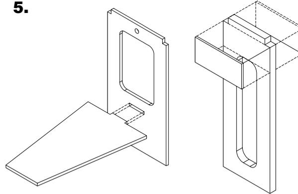
Glue the Liteply battery tray to the Liteply fuselage former F2 as shown. The angle between the two pieces should be 90 degrees. Also glue the 1/16" plywood doublers to the top of F4.
