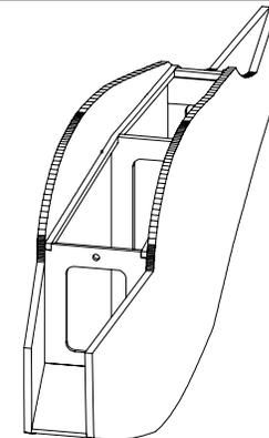
When the glue on formers F3 and F4 as fully set, pull the sides together at the nose so they are in contact with the battery tray. Glue the sides to the tray.
