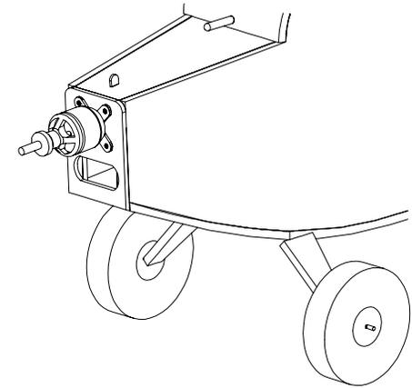
Mount the motor to the firewall. This is a good time to also mount the ESC and receiver.
