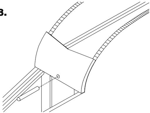
From the back side of F2, use a 3/16" diameter drill to make a hole in F5. Slide the 1 1/2" length of dowel through the hole so it fully engages F2. Glue the dowel to F2.
