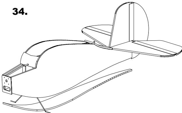
Glue the fuselage bottom to the fuselage assembly. Some pre-bending edge to conform to the shape will make this step easier to complete.
