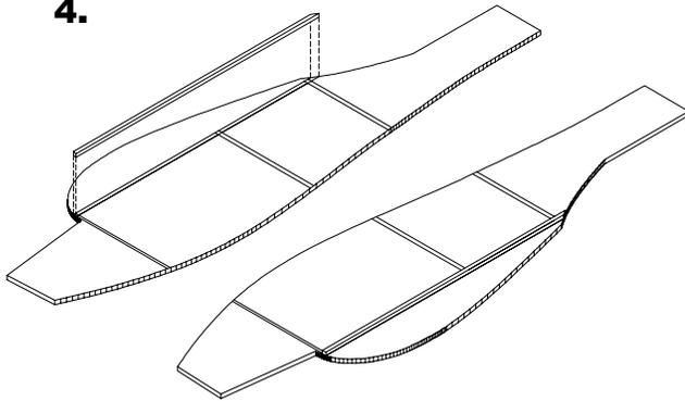
Glue 3/16" square balsa strips to the fuselage sides as shown. Use the reference lines as a location guide.
