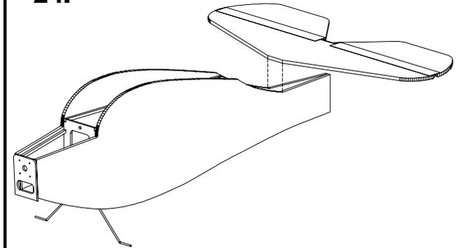
Glue the stab assembly to the fuselage as shown. Make sure it is square to the fuselage sides.
