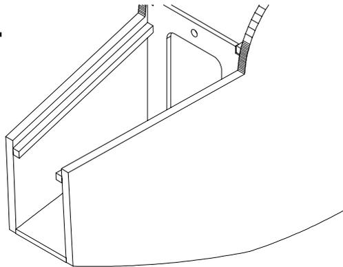
Using the marks as a location guide, glue 3/16" square strips of balsa to the inside face of each fuselage side as shown. These strips form the supports for the battery hatch.
