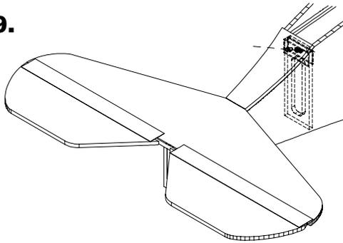
Make a mark 13/16" down from the top edge of the rear fuselage top piece. The mark should be centered on the top piece. Using a 3/16" diameter drill, drill a hole at the mark with the drill about 60 degrees down from vertical. You want to drill through F4 and the 1/16" plywood doublers on the top of F4.
