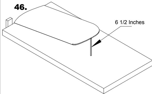
Place each wing panel at the edge of the work surface. Raise the tip 6 1/2 inches from the surface. Sand the root face of each panel so they are vertical.
