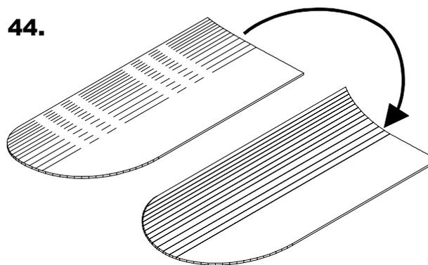
Use the crease lines on the wing panel template to bend the wing panels slightly at each crease line. A yard stick or something similar can be used when bending the panels. This pre-forms each wing panel to the approximate airfoil profile.
