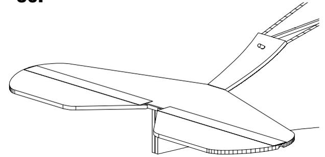
Slide the 2" length of dowel through the hole and also through the hole in the top of F4. Glue the dowel to F4.
