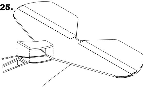
Glue the top rear fuselage piece to the fuselage assembly. Some pre-bending will help with this step. It may be necessary to sand the rear edge of this piece to be vertical.
