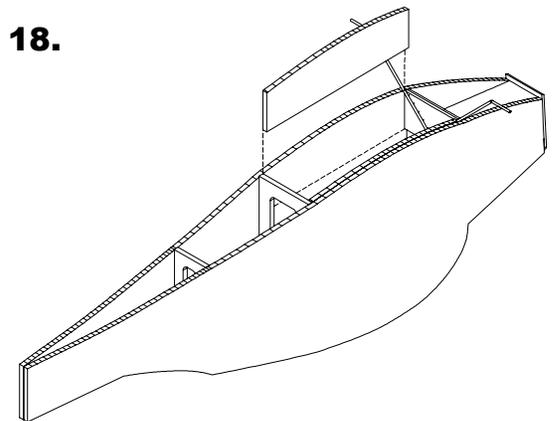
Glue the receiver/servo tray supports to the fuselage sides. They fit between F2A and F3.
