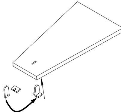
Assemble the 1/16" plywood hatch pull parts. Slide the hatch pull through the hole in the hatch from the bottom and glue it in place.
