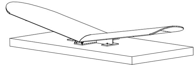
Use the same procedure as in step 50 for the right wing panel. Apply glue to the center joint before it is closed as the wing panel slides into position. Glue the wing panel and skewers to the center section assembly.
