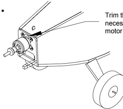
Trim the top block if necessary to clear the motor
