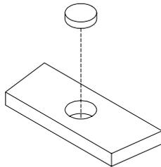
Glue a 1/4" x 1/16" magnet in the hole of F6. The magnet should be flush with one side of F6. Orientation of the magnet does not matter.
