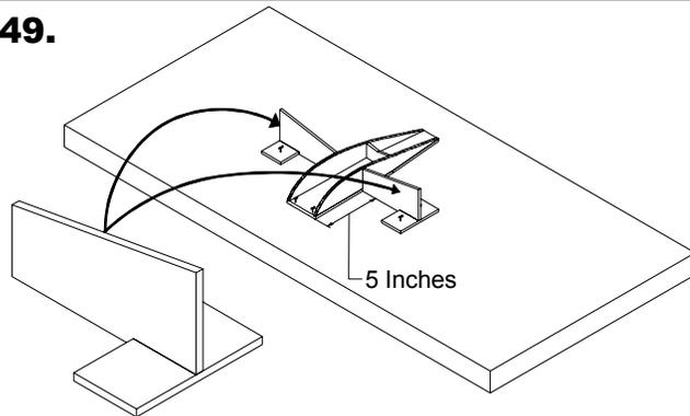
Assemble the two dihedral jigs. Pin the wing center section assembly to the building surface. Pin each dihedral jig to the building surface so they are touching the center section assembly 5" from the forward edge as shown.
