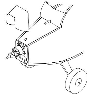
Glue 1/4" square pads of the hook and loop material to the outside face of each block. Glue 1/4" square pads of the opposite side of the hook and loop material to the inside face of the cowl at the block locations. Mount the cowl. It fits over the edge of F1.
