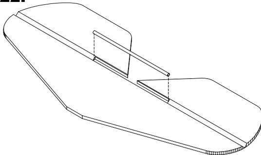
Cut a length of 3/16" aluminum tubing to a length of 6 1/2". Rough the surface with some sand paper. Lay the elevators next to the stab. Using epoxy, glue the aluminum tube jointer to the elevator halves. Remove the stab before the epoxy sets.
