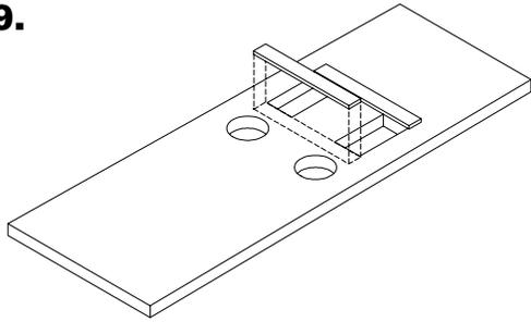
Glue some 1/16" plywood cut into 1/4" wide strips, or some 1/16" x 1/4" Bass wood to create hard points on the fore and aft edges of the servo cut outs in the receiver/servo tray. Mount the servos on the tray. Route the servo leads through the round holes in the tray.
