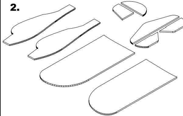
Cut out all of the parts. Note the parts that are to be cut from plywood rather than foam board.
