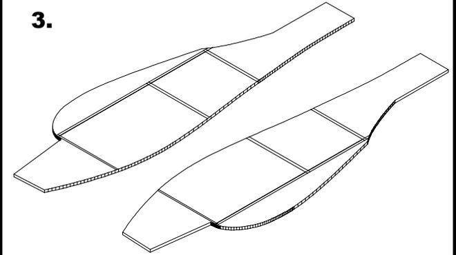
Using the fuselage side template, draw the template reference lines on each fuselage side. Be sure to make a left and right side.
