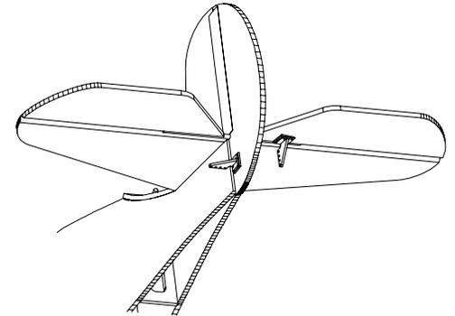
Install the rudder and elevator control horns. Use 1/16" plywood pads under the horns and locking plate. Determine the push rod routing for your specific servo installaton. Cut holes/slots in the fuselage sides for the pushrods. Install the pushrods. Use supports for the pushrods.
