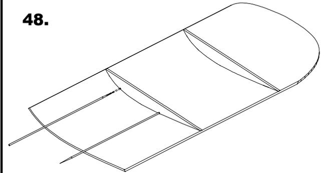
One end of each skewer has a sharp point. Use the pointed end to push the skewer through the first W2 rib. Remove the skewer and turn it around. Re-insert the skewer in the hole of W2 using the blunt end this time. Glue the skewer to the wing panel. Repeat the process for all of the reinforcement skewers.
