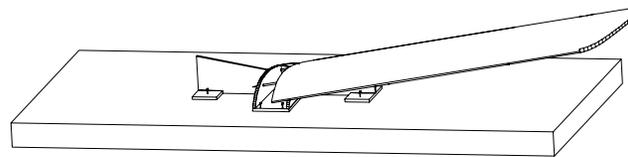
Slide the left wing panel along the dihedral jig until the ends of the skewers contact the W1 center section rib. Push the wing panel far enough to have the skewers pierce the W1. Push the panel until the root edge is centered over the center section assembly. Glue the wing panel and skewers to the center section assembly.
