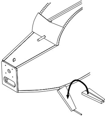
If desired, mount landing gear leg covers to the landing gear legs. Cut a slot in the back side of each over and then glue them to the legs with epoxy. Allow some clearance at the top between the fuselage sides for flexing of the legs.
