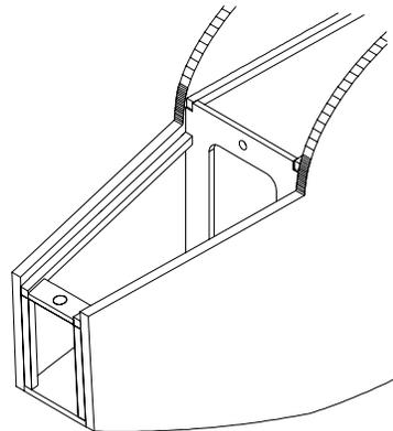
Orient F6 so the magnet is facing up. Glue F6 to the balsa hatch supports as shown. It lines up with the bottom edge of the supports. Carefully sand the nose so everything is flush with the sides.
