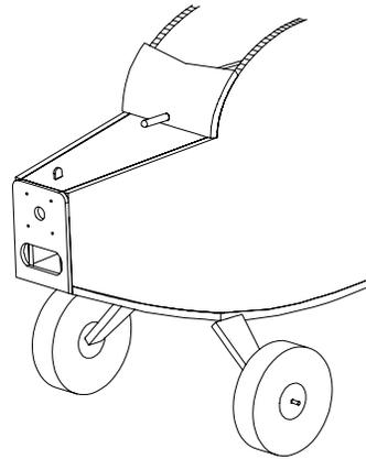
Mount 3" diameter lite wheels on the landing gear legs using 3/32" wheel collars.
