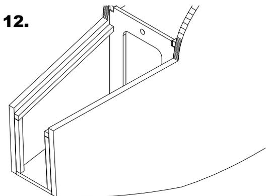
Glue a piece of 3/16" square balsa strip to the inside face of the nose of each fuselage side. The pieces fit between the battery tray and battery hatch supports.
