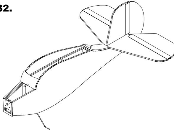
Glue the fin/rudder assembly to the top of the stab.
