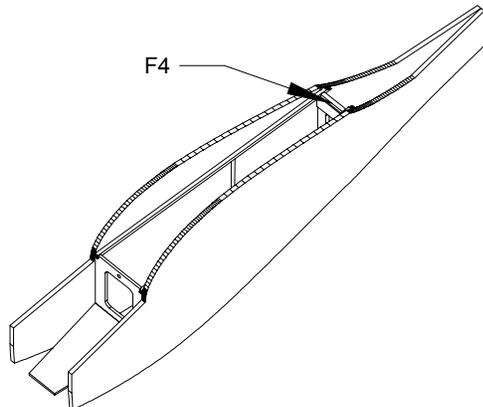
Glue fuselage former F4 in place. Use the drawn reference lines as a location guide.
