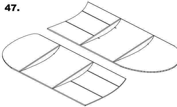
Mark the location of the bamboo skewer reinforcements on each wing panel. Note that the skewers on the right panel should touch the inside faces of the left panel skewers.
