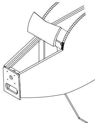
Glue part F5 to the forward edge of the wing mount area as shown.
