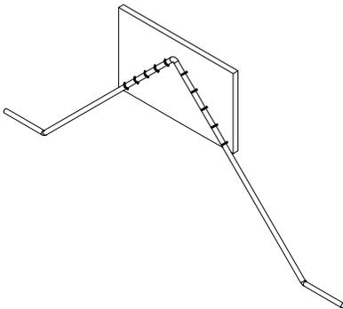
Make up the landing gear legs from 3/32" piano wire using the provided pattern. Bind the landing gear legs to F2A. The provided template shows the suggested location and associated 1/32" diameter holes to use with the binding material.
