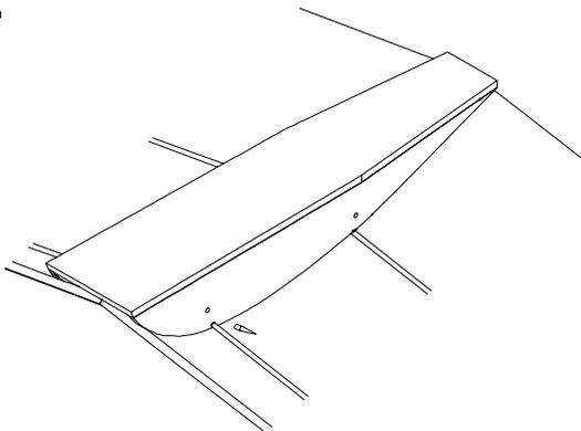
Trim off the excess skewer lengths on each side of the center section assembly.
