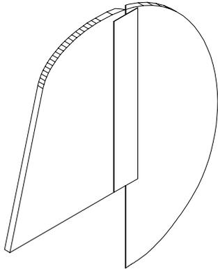
Like the stab and elevators, sand the trailing edge of the fin and leading edge of the rudder to a bevel. Attach the rudder to the fin using a piece of packing tape cut into a 1" wide strip.
