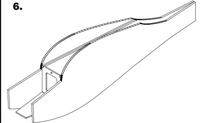
Glue the Liteply fuselage former F2 to each fuselage side as shown. Also glue the rear fuselage joint. The battery tray faces forward.
