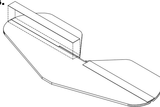
Cut some 1" wide strips of clear packing tape. Use the strips to attach the elevators to the stab.
