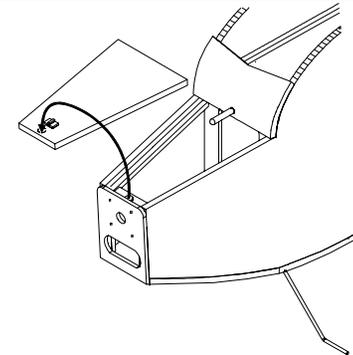
Place a 1/4" x 1/16" magnet on top of the magnet in the forward hatch support. Use a marker to mark the face of the magnet. Place the hatch on the model. Some marker ink will transfer to the hatch. Remove the hatch and glue the magnet in place with the marked face toward the bottom of the hatch.
