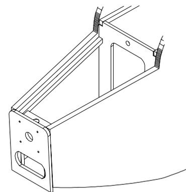
Mark the screw holes for the motor mount of your chosen motor on the 1/8" LitePly former F1. Drill pilot holes for the screws. Now glue the F1 to the nose of the fuselage as shown.
