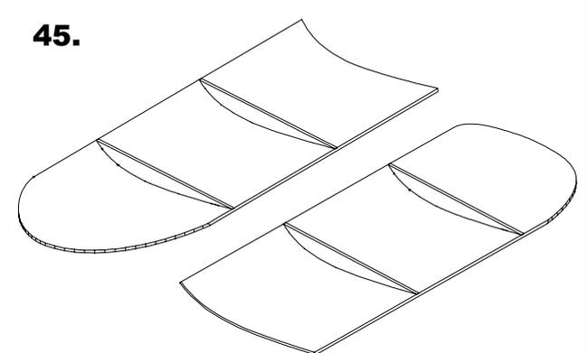
Glue ribs W2 to the wing panels. Use the reference lines on the wing panel template as a location guide.
