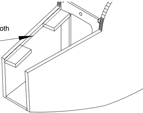
Use a scrap piece of the foam board to mark the depth of the battery hatch on the inside face of each fuselage side as shown.
