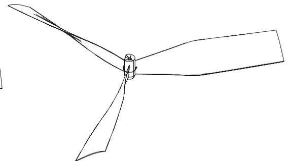
9. This completes the basic assembly of the prop. If the prop will not have a spinner, remove the plywood disk and file the brass tubing to be flush with the prop hub.
