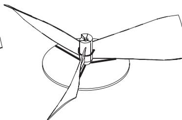
8. When the glue is set on the hub lashing, the free wheel ramp on the front of the prop assembly can be cleaned up with a file or Dremel style tool.
