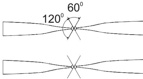
2. Using a razor saw, or other suitable cutting tool, cut each prop hub as shown. The included angle is 120 degrees or as close to that as you can eye ball. The angle can be a little off without causing a problem.
