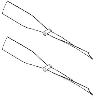
1. Select two identical props of the desired diameter. Drill the prop shaft hole in each prop to 1/16" diameter.
