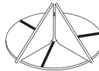
5. Glue a length of 1/16" diameter (OD) brass tubing in the center hole of the disk. Use triangles to make sure the tubing is perpendicular to the plywood disk. The triangles are not glued to the assembly. Remove them when the tubing is in place.
