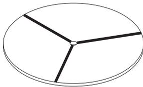
4. Make a disk from 1/32" plywood. If your prop will have a spinner make the disk the diameter of the spinner. Drill a 1/16" diameter hole in the middle. Mark the disk with three lines spaced 120 degrees apart. Be accurate here.
