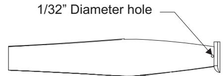
3. Set aside one blade for a future prop. Drill a 1/32" diameter hole in the middle of each remaining blade next to the hub.
