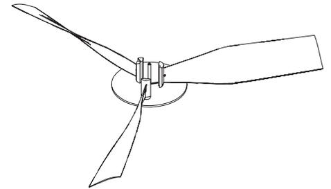
6. Glue each prop blade to the brass tubing using the lines on the disk as alignment marks. Don't worry if the hub joint is not perfect.
